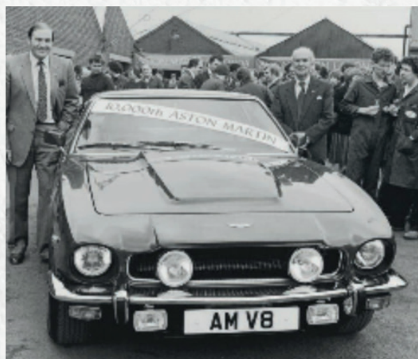
A 0-60 mph time of 5.2 seconds and a top speed approaching 170 mph made the V8 Vantage not only the UK's first true supercar but also the fastest 4 seater production car in the world.
